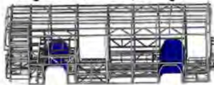
Original structure 2,877 Kgs.
